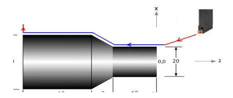
N010G28U0.0W0.0; N020G92S2500; N030T0101; N040G96S150M04; N050G00X57.0Z2.0; N060G73U1.0R1.0; N070G73P40Q50F0.2; N080G01X25.0Z0.0; N090Z-60.0; N100G00X57.0Z2.0; N110G28U0.0W0.0; N120M30;
