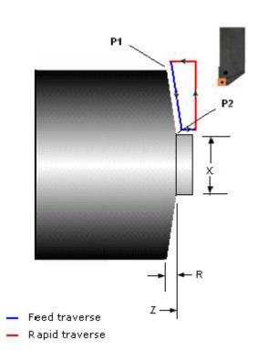
Format G94 X\_ Z\_ R\_ F\_ X = X coordinate of end point of cut Z = Z coordinate of end point of cut R = Taper amount
