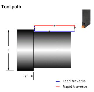
Format G90 X\_ Z\_ F\_ X = X coordinate of end point of cut, absolute
